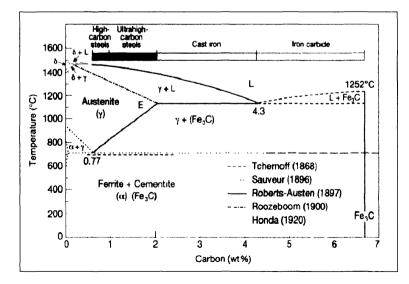
Figure 2. Iron-carbon (Fe-C) diagram (first phase diagram of any alloy to be established, by Roberts-Austen in 1898 after whom austenite came to be named.).
