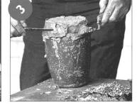
Seal the loaded crucible with putty.
