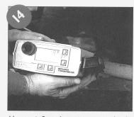
Use an infrared pyrometer to check the temperature of the steel. As the steel cools, the color of the metal changes, too.
