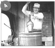
Put the crucible into the kiln.
