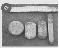
The different shapes the steel cake takes after it's been heated, stretched, and hammered for a blade.
