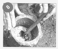
Remove the crust to reveal the steel cake.
