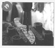
Use a drill to make one-tenth-of-aninch-deep holes on both sides of the blade. This is where the rose pattern will appear.
