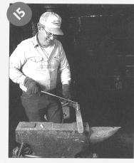
Use a magnet to test the steel. The metal's magnetic field changes as it cools. It won't attract the magnet when red-hot. Make chalk marks on the anvil to keep track of how many times the steel's been hammered and returned to the fire.
