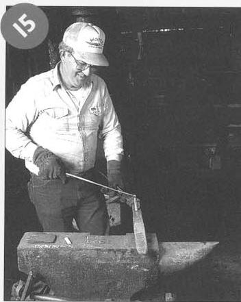
Use a magnet to test the steel. The metal's magnetic field changes as it cools. It won't attract the magnet when red-hot. Make chalk marks on the anvil to keep track of how many times the steel's been hammered and returned to the fire.
