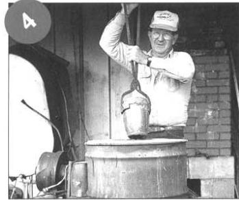
*Put the crucible into the kiln.*
