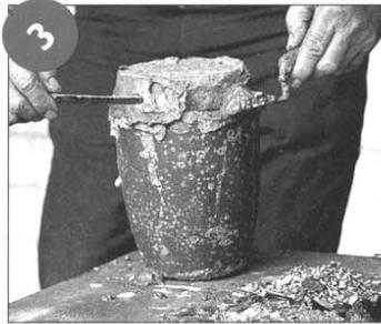
*Seal the loaded crucible with putty.*
