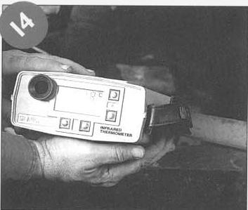
14 Use an infrared pyrometer to check the temperature of the steel. As the steel cools, the color of the metal changes, too.
