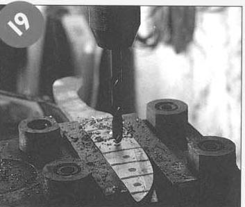
19 Use a drill to make one-tenth-of-an-inch-deep holes on both sides of the blade. This is where the rose pattern will appear.
