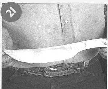
21 Reheat, rehammer, and regrind your blade. No cuts or holes should show.
