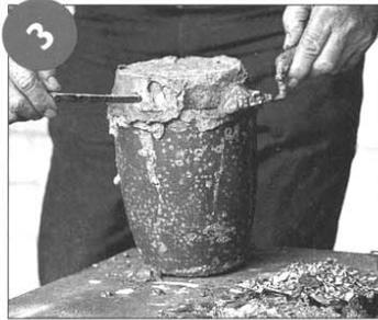
*Seal the loaded crucible with putty.*
