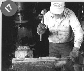
*Cut the steel short to form a knife blade.*
