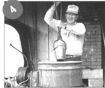
*Put the crucible into the kiln.*
