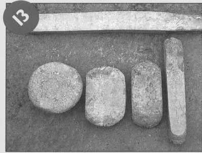
*The different shapes the steel cake takes after it's been heated, stretched, and hammered for a blade.*
