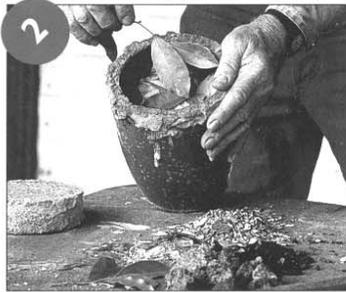
*Load the ingredients into a crucible.*
