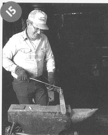
15 Use a magnet to test the steel. The metal's magnetic field changes as it cools. It won't attract the magnet when red-hot. Make chalk marks on the anvil to keep track of how many times the steel's been hammered and returned to the fire.
