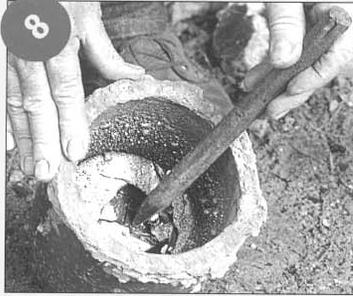
8 Remove the crust to reveal the steel cake.
